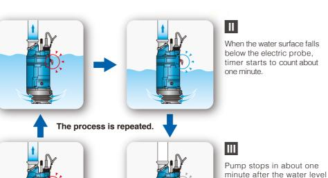
When the water level rises to contact the electric probe, pump starts operating again.
